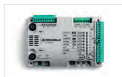
Scheda elettronica 1/2 motori 230V HP Electronic control 1/2 motors 230V HP
