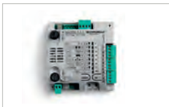
Scheda elettronica 2 motori 24V Basic Electronic control 2 motors 24V Basic
