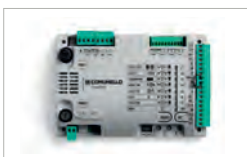
Scheda elettronica 1/2 motori 24V HP Electronic control 1/2 motors 24V HP
